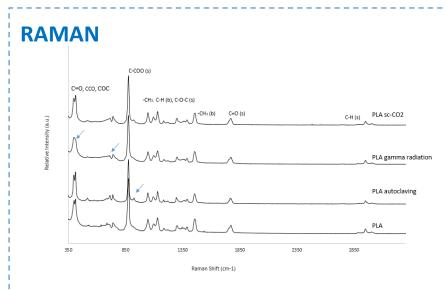
Autoclave sterilization and gamma radiation cause minor changes in some of the Raman bands
