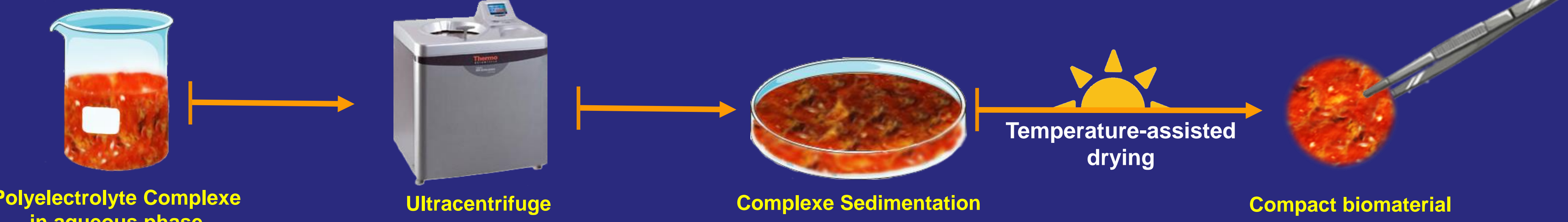
Figure 4. Schematic representation of the compaction procedure by centrifugation. The process compacts the polymers and removes the wastewater, create a biomaterial membrane.
