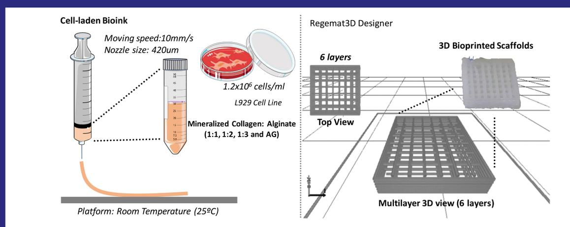
Figure 1. Schematic representation of the process to fabricate cell-laden mineralized collagen:alginate hydrogels by using a Regemat3D printer dispensing system.
