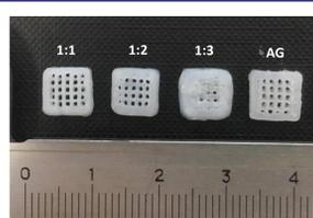
Figure 5. Photograph of the printed hydrogels: from left to right, decreased concentrations of mineralized collagen
