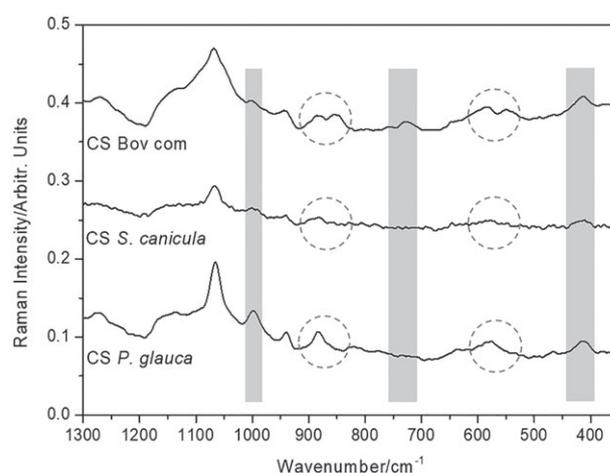
**FIGURE 4** Raman spectra in the wavenumber range of interest (1,300–350  $\text{cm}^{-1}$ ) obtained for chondroitin sulphate from *Scyliorhinus canicula* in comparison with chondroitin sulphate (CS) Bov com (4-sulphate prevalence) and CS *Prionace glauca* (6-sulphate prevalence)
