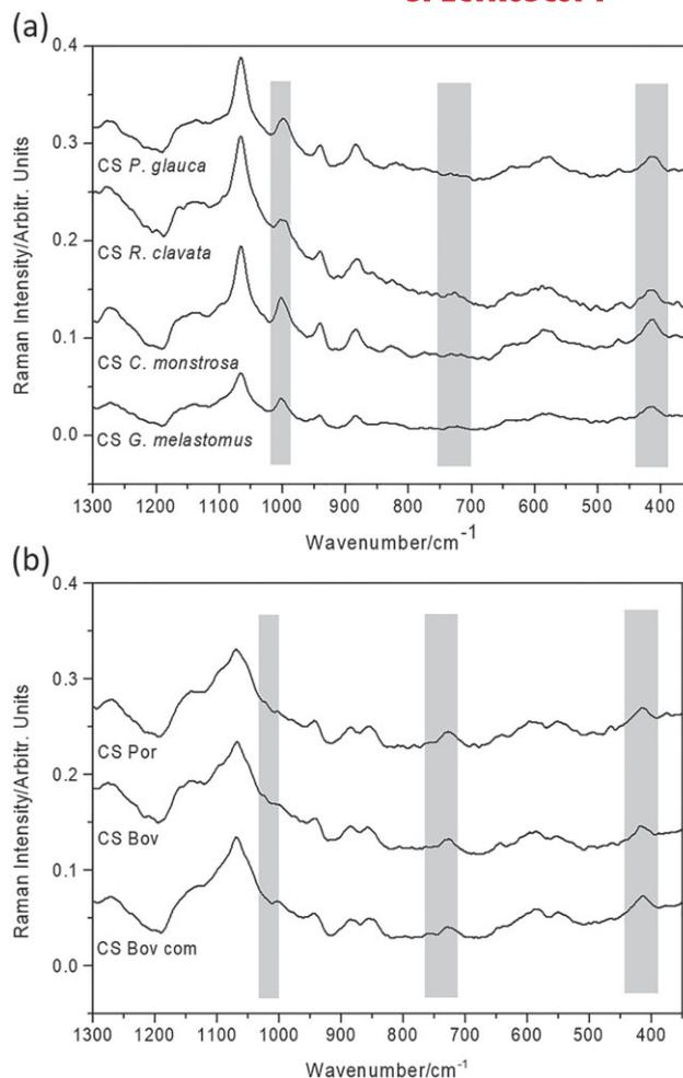
**FIGURE 2** Raman spectra in the wavenumber range of interest ( $1,300\text{--}350\text{ cm}^{-1}$ ) obtained for the whole series of chondroitin sulphate of fish sources (a) and of mammalian sources (b)
