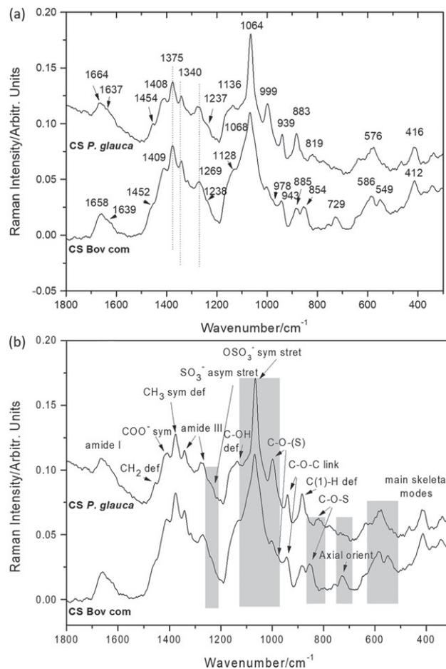
**FIGURE 1** Raman spectra of representative chondroitin sulphate (CS) *Prionace glauca* from fish source and CS Bov com (commercial bovine CS) from mammalian source in the wavenumber range of 1,800–350  $\text{cm}^{-1}$  (a). Corresponding attributions with bands directly related with sulphate group vibrations or specific orientation of the isomers highlighted in grey (b)
